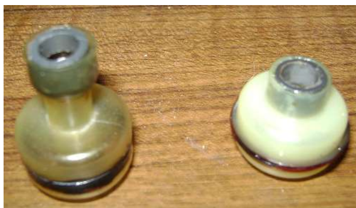
Two types of reservoir float. The ring magnets can be seen clearly. The floats rarely leak but it is worthwhile checking them.
