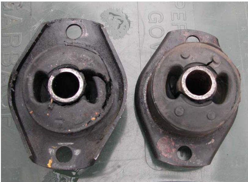
These grotty things are the caster bushes that stop the front wheels falling over . Simple to replace, they seem to last 60 – 90K and can be replaced without disturbing the wheel alignment.
