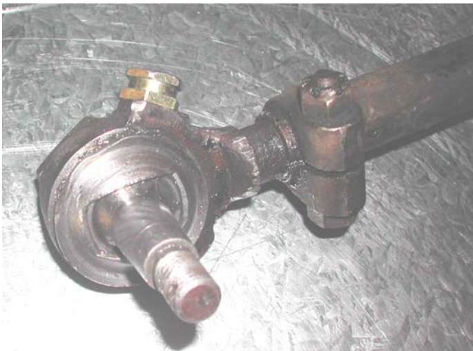
The outer ball joint on a Shadow with its rubber cover off. Note the dented lip on the top side from someone using the bashing method of tie rod end joint extraction.
