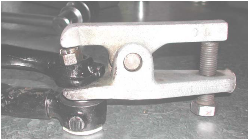
The preferred method. These scissor type removers are readily available and utterly reliable.
