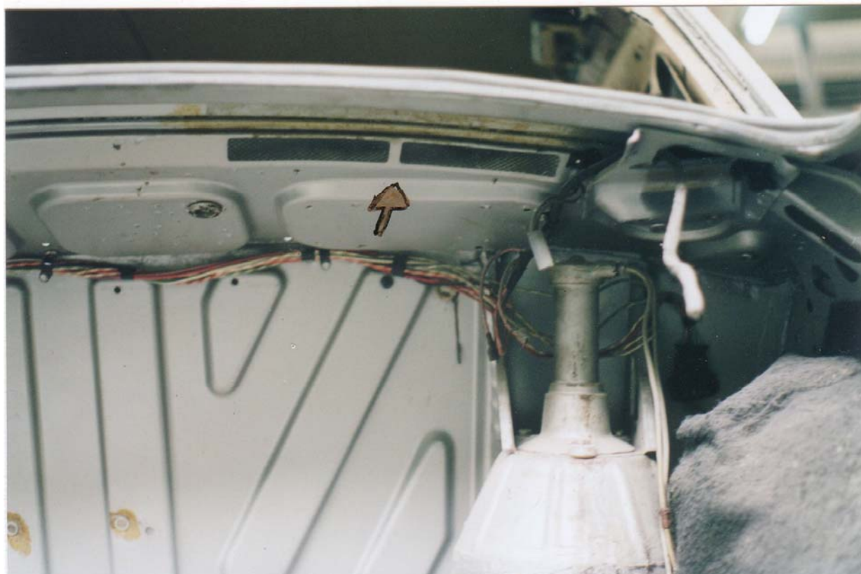
A view many owners would not have bothered to find. To the right is one of the oft discussed rams on which the rear of the car rides. The arrowed slots however are a later improvement allowing air flow through to the boot which helped the sealing in the later and the minimisation of dust entry. Courtesy Nick Lang.
