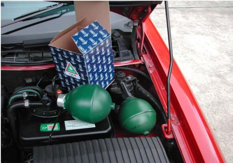
Doug's Spirit. Dimensionally they were identical as were the charged pressures. Apparently the spheres differ throughout the Citroën by the use of restrictors in the neck of the unit which are swaged in. The other difference is that the Citroën units are a third of the cost of the RR items! And the enthusiasts re-charge them!!
