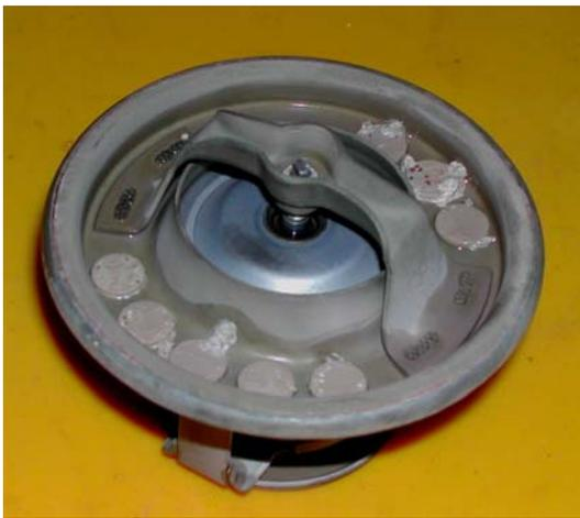
The plugs are fusible and melt at approximately 124°C if the temperature gets to that level or the thermostat fails. Thermostats are not adjustable and probably should be replaced about every two years. Never run an engine without one. They usually fail open which shows up on the
