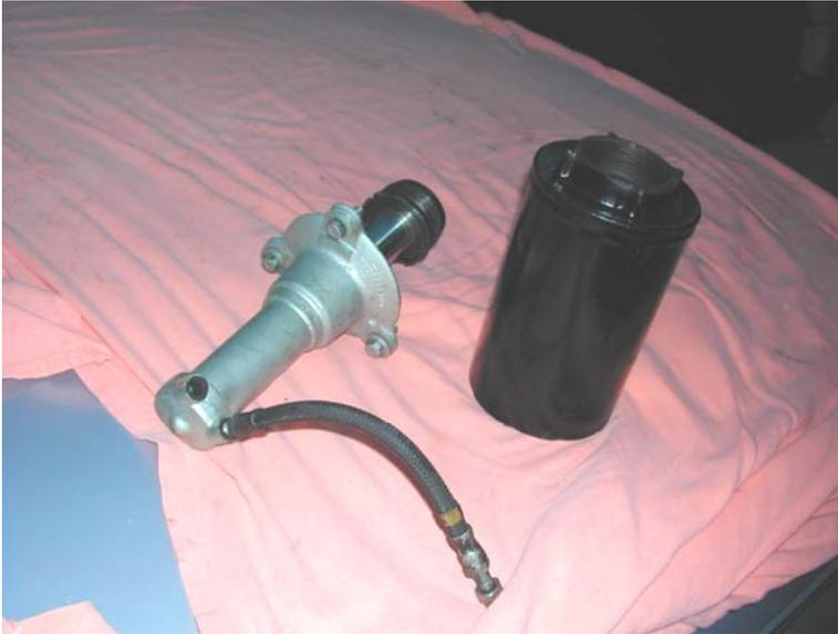
For those that have not seen them these are the gadgets that lift the rear of your shadow. The cylinder on the right screws onto the ram and in turn sits on the road spring suitably separated by an isolator that insulates and locates the coil. It also allows shims to be placed above the spring to adjust the height.
