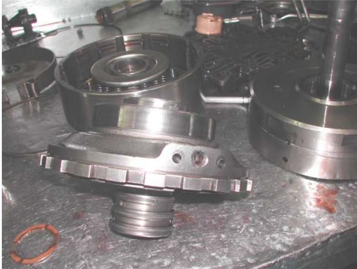
Examination of the main casing showed that the area where the above retaining bolt passes through the box was significantly distorted most probably through over tightening. This allowed the central carrier to move around in the box losing oil pressure to the front clutch and allowing
