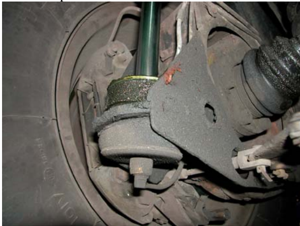
Spirits rely heavily on their rear shock absorbers and level the car from the number 2 system. Here is a common problem a leaking lower seal evidenced by the wet upper rubber bush
