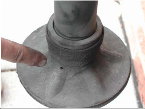
Where the holes are. There are three. Relax, you don't have to take the springs out to clean them.
