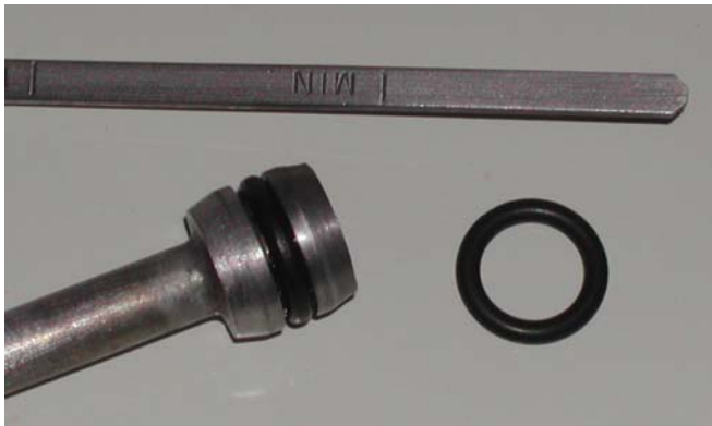
And here is a better picture of the business end of the dip stick and tube
