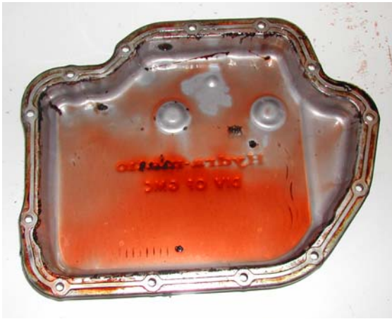
And here is a sight to delight any owner – a transmission sump without any nasties in it. The black spots are actually accumulations of transmission clutch dust a normal feature of any friction device.
